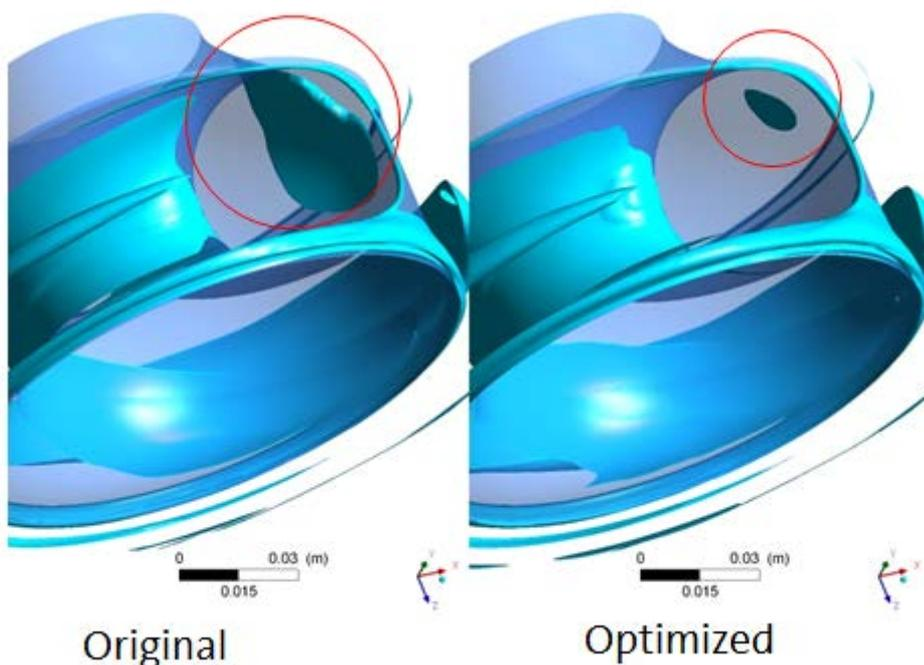
**Figure 3:** In this multiphase CFD simulation, the two impellers are of similar size but slight geometric difference (within a few millimetres) in shape. The fluid flow is the same for both impellers, with 8 per cent air continually added to the flow. The circled areas show the accumulated air bubbles in each and how air handling may be optimised by specific design.
